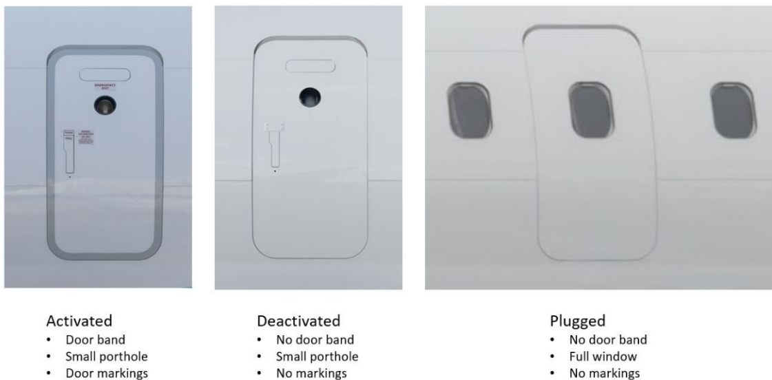
Figure 3. Three types of mid exit doors. (Source: Boeing. Image Copyright © Boeing. Reproduced with permission.)
